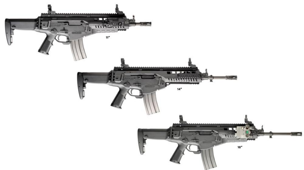
**Product:** The automatic rifle ARX 160 consists of a rifle and a 30 rounds magazine cal. 5.56 x 45 mm NATO. The rifle may be configured with barrel lengths of 11, 14 and 16 inches, respectively; ARX 160 features a quick-change barrel, so that to be removed and installed in a few seconds without tools. It is a gas-operated, locked breech rotating bolt weapon, that can be fired either in burst or single shots.
