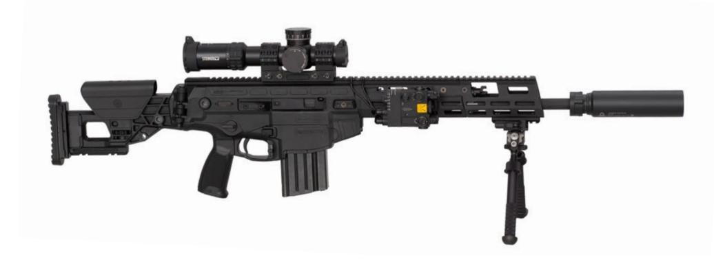
**Product:** The automatic rifle ARX 160 consists of a rifle and a 30 rounds magazine cal. 5.56 x 45 mm NATO. The rifle may be configured with barrel lengths of 11, 14 and 16 inches, respectively; ARX 160 features a quick-change barrel, so that to be removed and installed in a few seconds without tools. It is a gas-operated, locked breech rotating bolt weapon, that can be fired either in burst or single shots.
